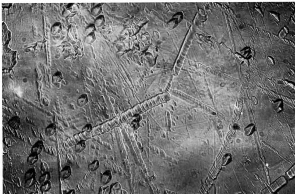
Fig. 6. Rhombohedral cleavage face etched for 15 min in sodium hydroxide solution ( \times 175 ).
