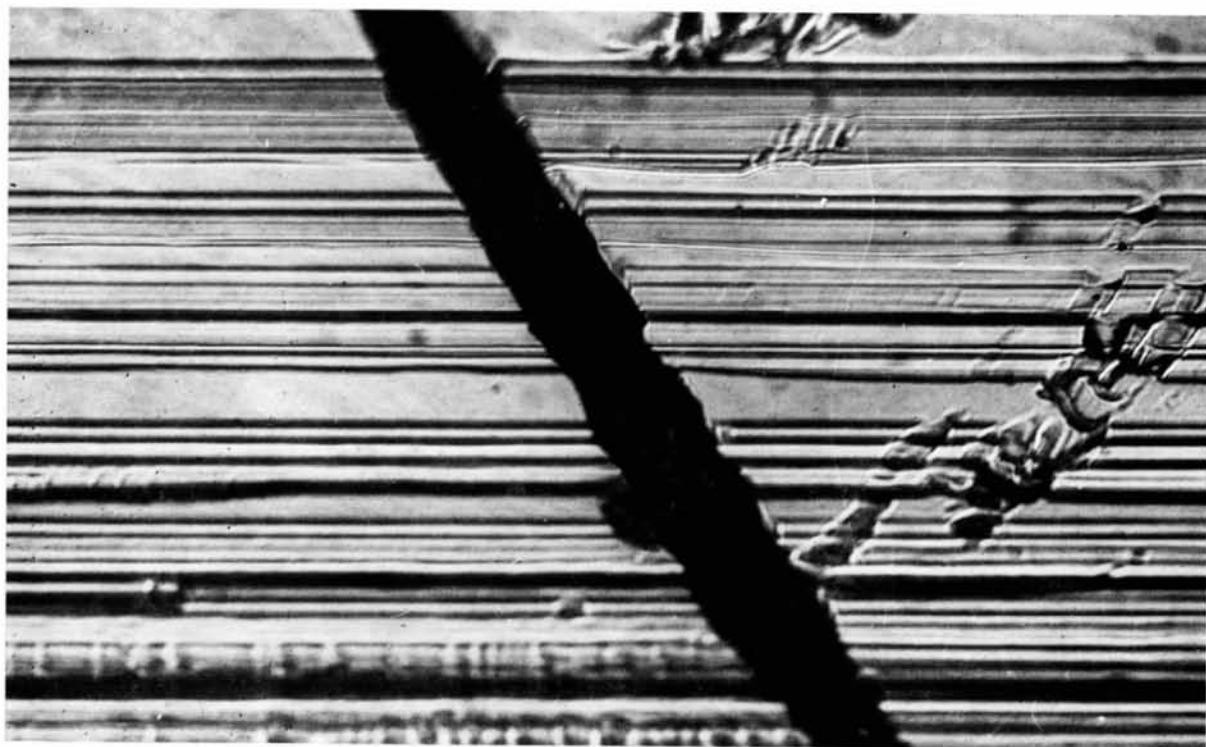
Fig. 8. Natural quartz crystal cleaved along a rhombohedral plane and etched in sodium hydroxide solution ( \times 250 ).
